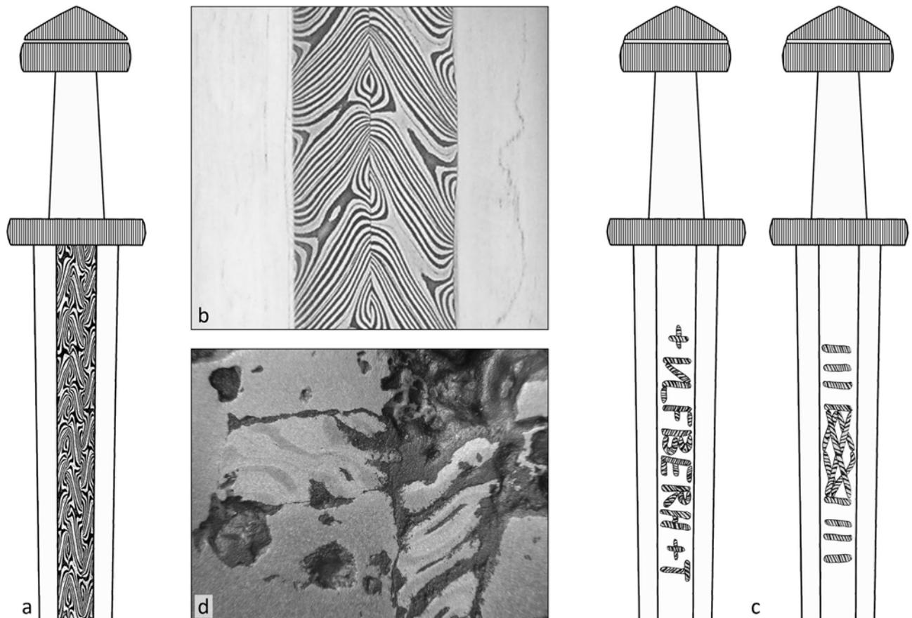
Fig. 1: Pattern welding and possibilities of its application to historical sword blades: a – pattern welding in the central part of the blade; b – an example of the real appearance of a pattern welded blade (modern replica made by P. Bárta); c – pattern welding applied in the form of an inlaid inscription and motives; d – an example of the real appearance of an inlaid pattern welded cross found on an archaeologically excavated blade
